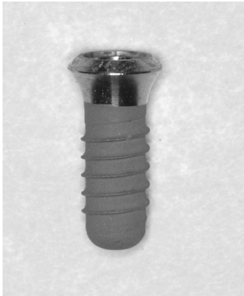
Figure 6.9 As an alternative to dentures, patients can have metallic dental root prosthetics implanted to replace each missing tooth. The implant is then topped with a porcelain crown. One advantage of dental implants over dentures is that the implant transmits mechanical forces into the jaw bone and stimulates it, resulting in less bone recession over time. (Photograph courtesy of Dr. Martin Freilich of the University of Connecticut Health Center.)
