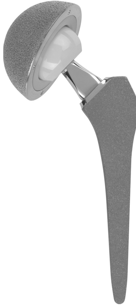
Figure 6.10 In this artificial hip joint, the polymer bearing surface and some of the metallic components have been replaced by ceramics to improve the durability of the joint replacement. This design features a ceramic femoral head and acetabular cup. (Photograph of the LINEAGE ® ceramic-ceramic acetabular cup system is courtesy of Wright Medical Technology, Inc.)
